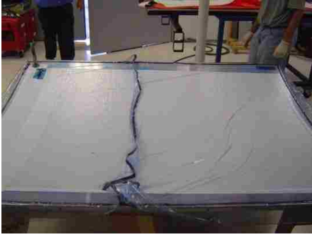
Figure 3-10: Skin Layup Bagged and Being Debulked
