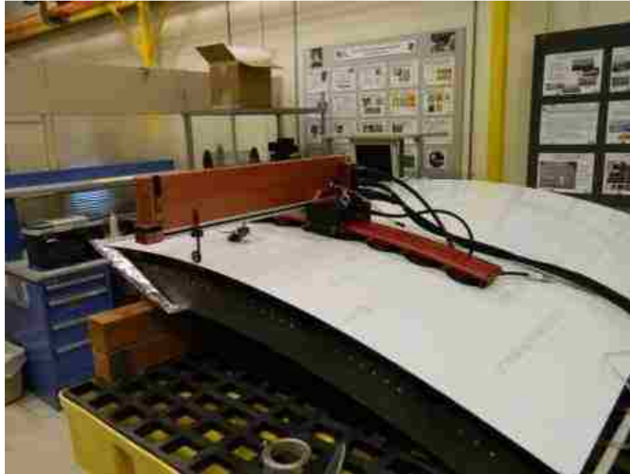
Figure 4-2: Boeing MAUS V Scanning System Conducting a UT Inspection
