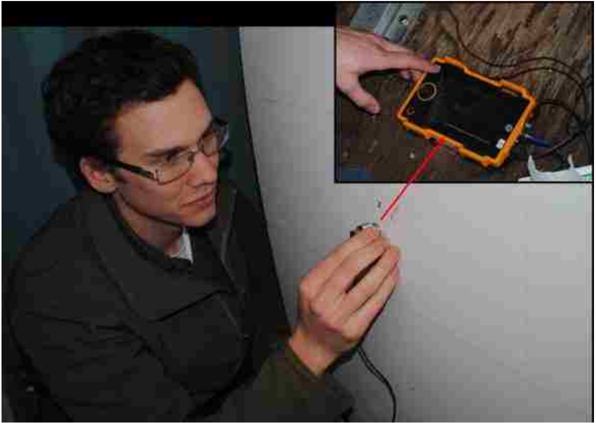
Figure 3-22: Ultrasonic A-Scan Inspection Being Performed After Impact to Determine Damage Extent
