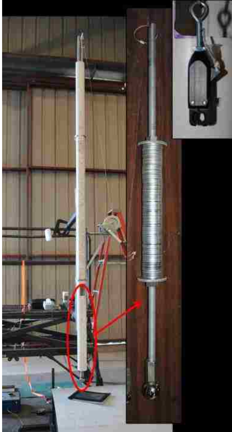
Figure 3-25: Guide Tube, Drop Spear with 2” Diameter Impact Tip and Quick Release Mechanism
